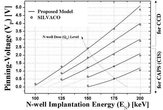
Fig. 2. Plot of the Pinning-voltage( $V_p$ ) vs. N-well implantation energy( $E_N$ ) of the proposed model in comparison with the simulated results for various cases of N-well Dose( $Q_N = 1 \times 10^{12} \text{cm}^{-2}$ ,  $2 \times 10^{12} \text{cm}^{-2}$ ,  $3 \times 10^{12} \text{cm}^{-2}$ ,  $4 \times 10^{12} \text{cm}^{-2}$ , and  $5 \times 10^{12} \text{cm}^{-2}$ ). Other conditions( $Q_p$ ,  $E_p$ ,  $P_{epi}$ ) are fixed.
