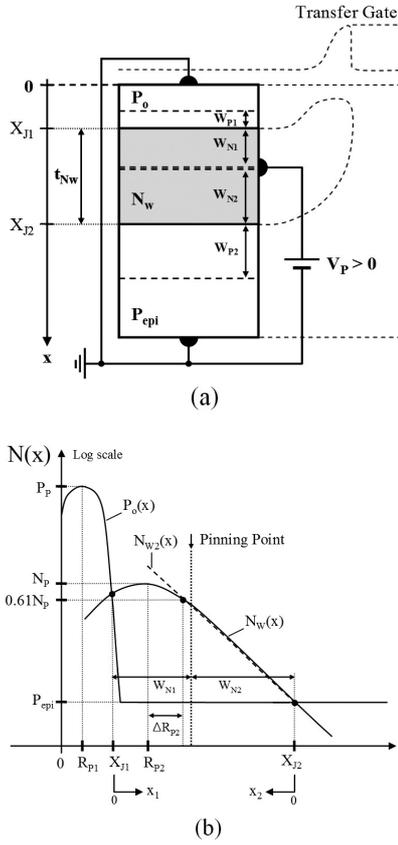
Fig. 1. (a) A schematic diagram in cross-sectional view and (b) doping profiles based on the Gaussian distribution of the PPD (where  $t_{Nw}$  is the junction thickness of the N-well,  $W_{N1}$  is the depletion width in the N-well region at the junction of the  $N_w/P_o$ , and  $W_{N2}$  is the depletion width in the N-well region at the junction of the  $N_w/P_{epi}$ ).
